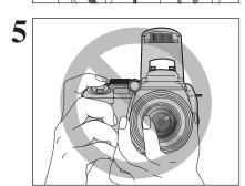
Hold the camera so that your fingers or the strap do not cover the lens, flash and AF-assist illuminator. If the lens, flash or AF-assist illuminator is obscured by your fingers or the strap, subjects may be out of focus or the brightness (exposure) of your shot may be incorrect.
