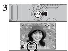
Position the subject in the center of the screen and press the "AE-L" button.
