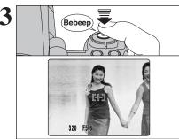
Press the shutter button down halfway (AF/AE lock). When a short double-beep is heard, the camera focuses on your subject. The AF frame on the screen becomes smaller and the camera sets the shutter speed and aperture. The indicator lamp (green) changes from blinking to lit.
